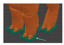
This option will generate a thin layer around the base of the model, which will improve the adhesion to the print bed. This is a handy option for models that don't have enough of a grip in proportion to their size.
