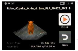
You will see a little preview of the model, and the estimated print time. Once you confirm by pressing the **Print** icon, both the print sheet and the nozzle will start heating up. No user input is needed from that point on – the printer will run through cleaning the nozzle, measuring the distance to the print bed, and preparing to print. During these steps, the heated nozzle may leak a bit of filament. It is normal and nothing to be concerned about.
