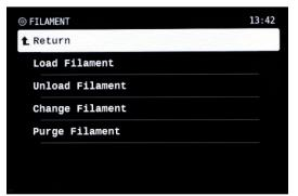
Here, you can **Load** or **Unload Filament**, **Change Filament** (which is just the two previous options one after another) or **Purge Filament** (i.e. get rid of the remnants of the previous filament color - normally, this is already included in the **Load Filament** procedure, though).
