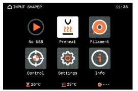
The upper right corner shows time, in the middle, there are 6 menu options, and at the bottom of the screen, you can see nozzle temperature, heatbed temperature, and type of material loaded into the printer. During a preheat, the temperatures will be in the format "current temperature/target temperature".
