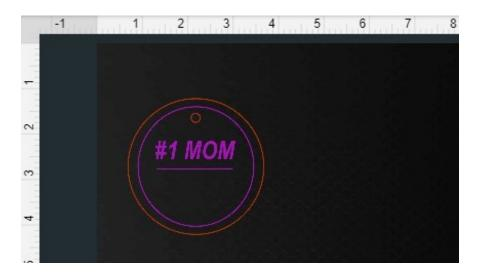
The interface will display the Glowforge bed. In this image there is no material loaded. The black honeycomb background is the crumb tray.
